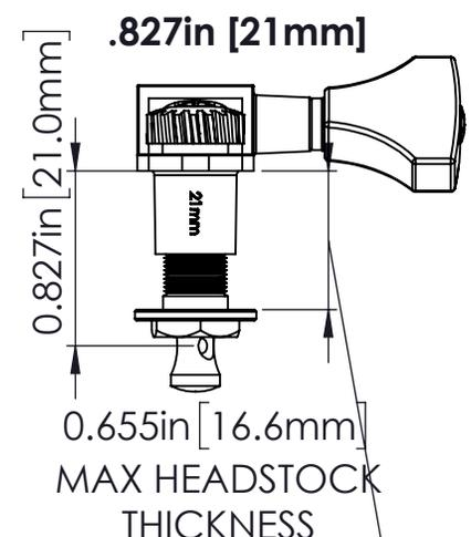
0.500in [12.7mm] MIN HEADSTOCK THICKNESS (SAME FOR ALL TUNERS)
